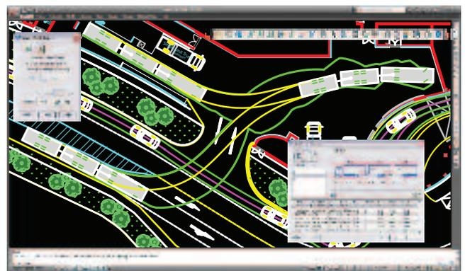
» Powerful features make vehicle reverse maneuvers easier than ever. Hatch vehicle body envelopes and swept paths to check for clearances.
